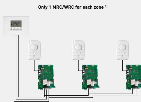
1) Up to 15 Plogic/fan coil units. Fan coil units can be of different types, with AC or EC fan motor.
